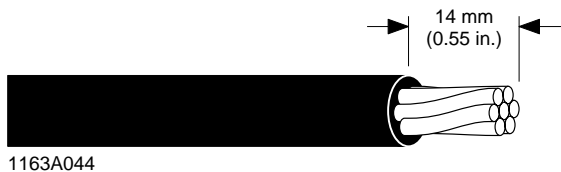
Figure 7. Phase Conductor and Ground Conductor Strip-length Requirement
